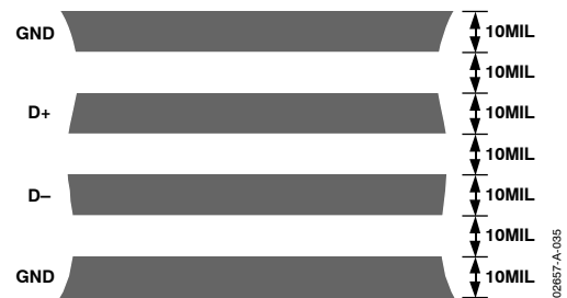
Figure 35. Arrangement of Signal Tracks
